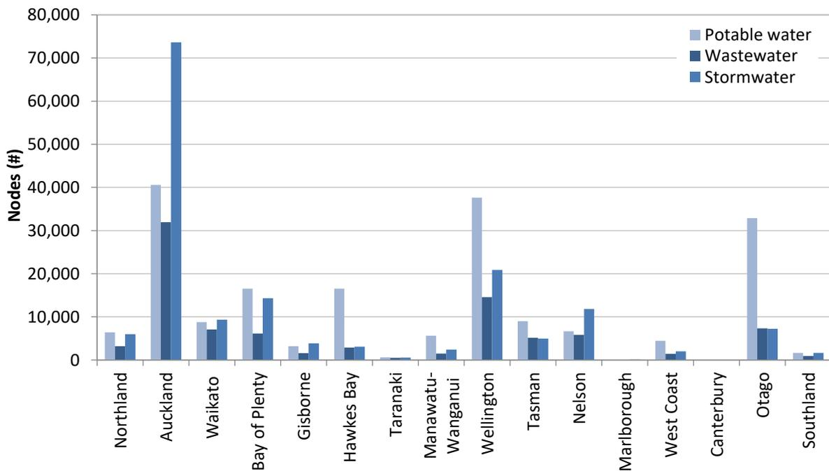
**Figure 3-15: Region level three-waters network node exposure in the FLHA map. Note: for this study, three-waters network node data was not available for Canterbury region, while limited data was available for Marlborough region.**
